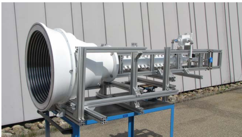
Picture shows Feed Network (without Diplexers) equipped with an S-/ X- Band Feedhorn for 15.5 m Cassegrain Antenna
